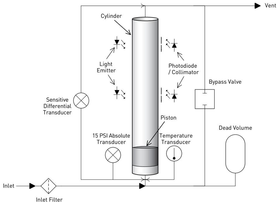
Figure 4 - Prover with Enhanced Dynamic Pressure Measurement
