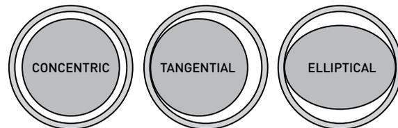
Figure 10 – Limit Cases of Equal Piston Area
