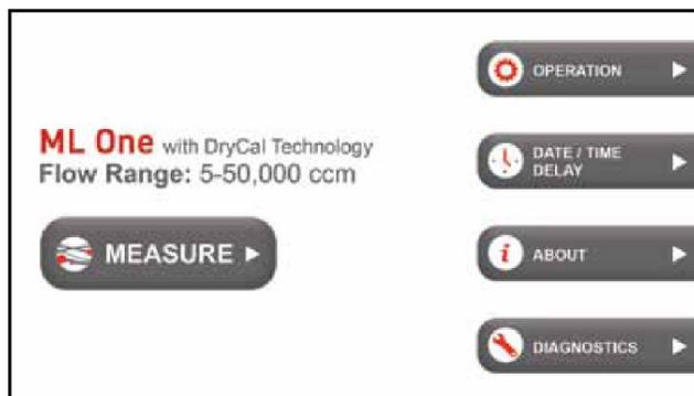
Touch to go to MEASURE, OPERATION, DATE/TIME DELAY, ABOUT or DIAGNOSTICS screen.
