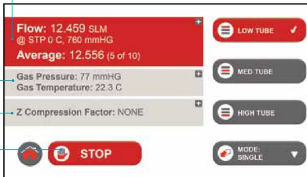
Touching selects the measurement tube. High Tube is default. The ML-One will auto change to a different tube if the flow is outside the tube's flow range.
