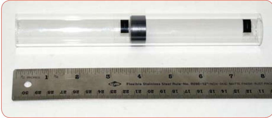
Figure 2 - Viscous-sealed piston/cylinder assembly
