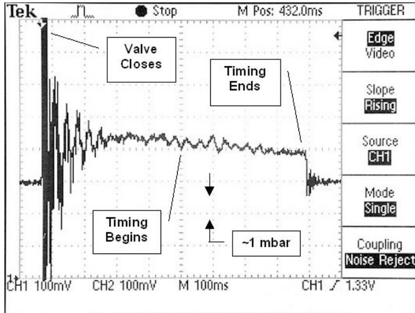
Figure 3 – Intra-Cycle Cell Pressure
