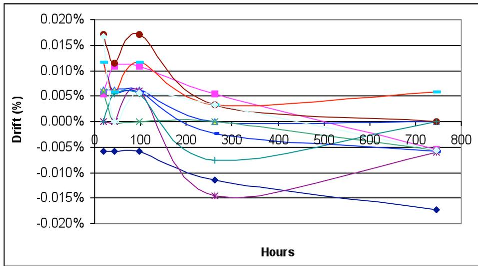
Figure 5 – Thermistor Drift
