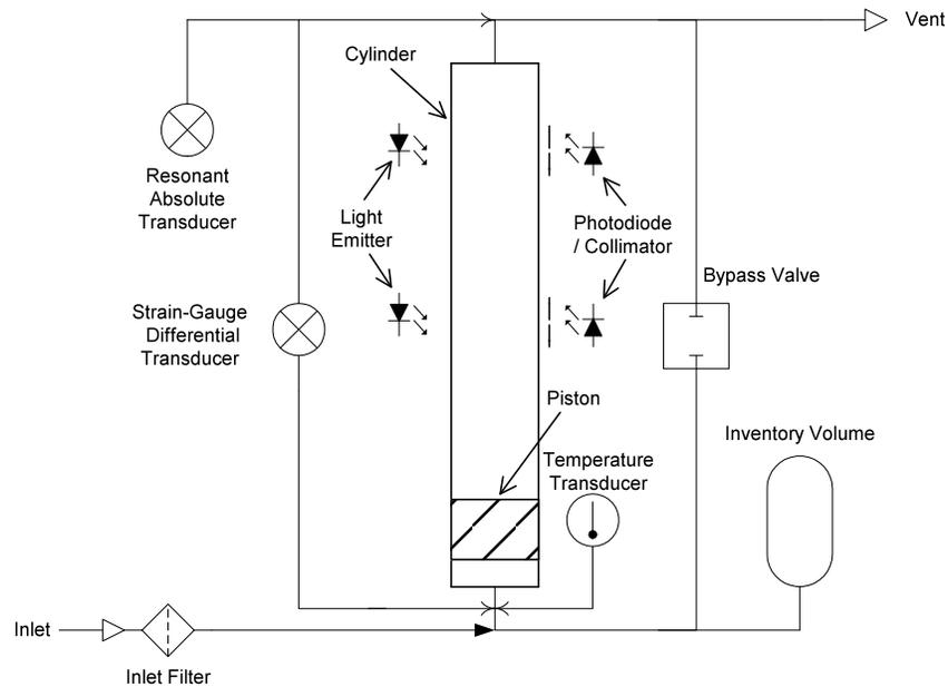
Figure 4 – Dual Pressure Transducer Variant
