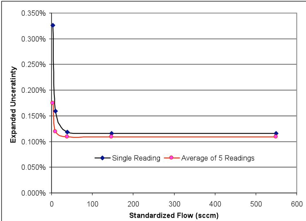
Figure 7 - Standardized ML-800 Small Cell Expanded Uncertainty (2X)
