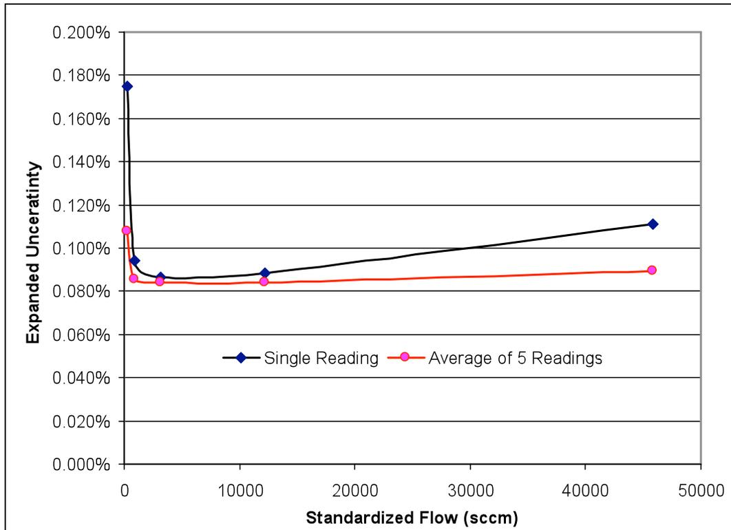
Figure 9 - Standardized ML-800 Large Cell Expanded Uncertainty (2X)
