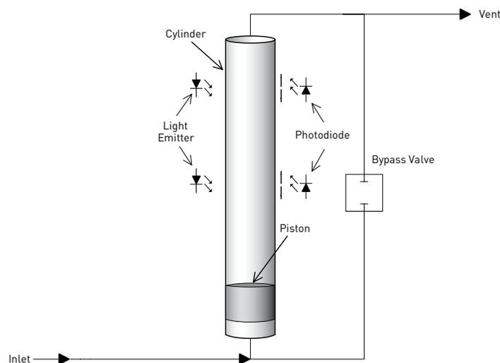
Figure 1 – Idealized Automatic Piston Prover
