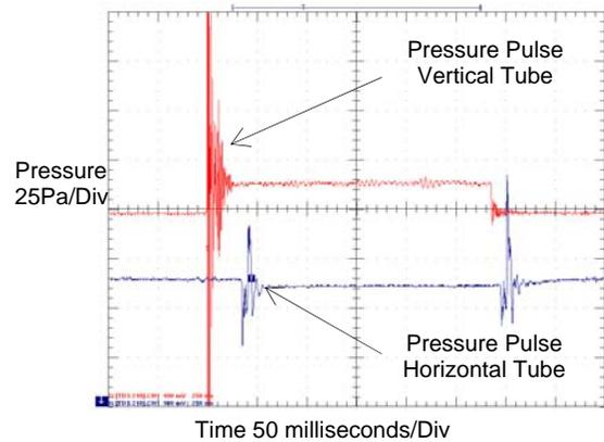
Figure 5: Piston Prover Pressure Pulse
