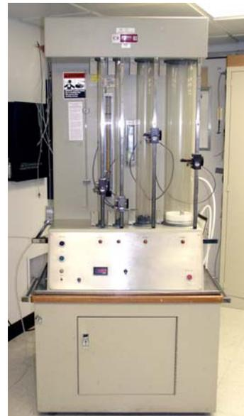
Figure 1: Mercury Seal Piston Prover
