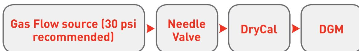
Follow the connection diagram below for a third party console such as Environmental Supply's Mercury Emissions Sampler. Connect the DryCal, DGM, and Flow source as shown in the connection diagram. Use the needle valve to create the pressure drop necessary to provide isolation and to simulate the mercury absorbent tube.
