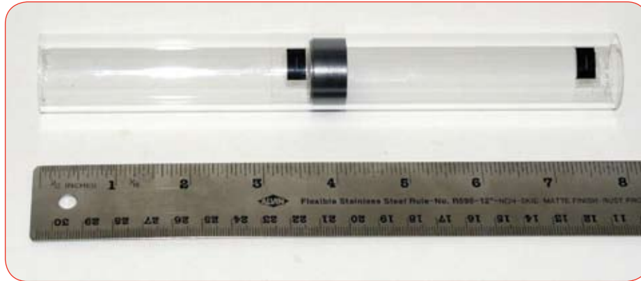
Figure 2 – Viscous-sealed piston and cylinder
