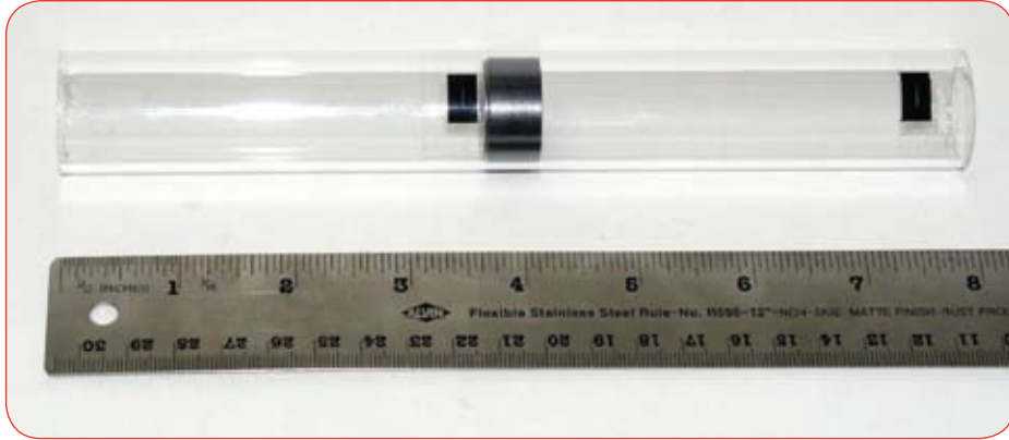
Figure 2 - Viscous-sealed piston/cylinder assembly
